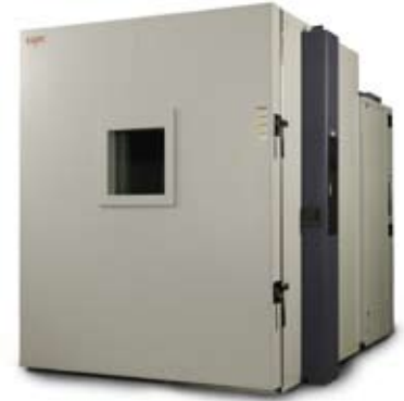
Solid walk-in chambers like this one are commonly selected for full-size solar panel testing.
