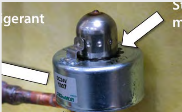
The needle valve in an ELV is opened by a stepper motor based on refrigeration demand by the chamber controller.
