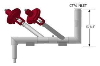
\* Optional Vacuum Jacketed Manifold for T1.5 and T2.0 Part number: 785-3171 factory installed 785-3206 field retrofit
