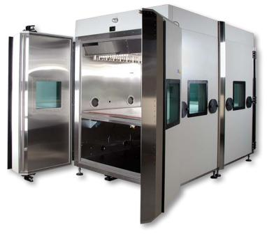
High Rate, High Flow T-series Thermal System
