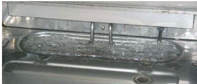
A humidity bath heats water right in the chamber for faster response and easier maintenance than traditional steam generators.
