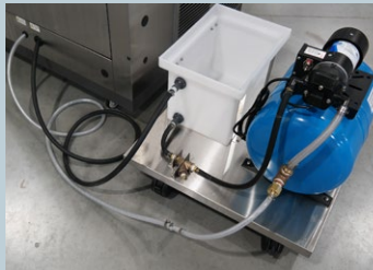
System has a recirculation mode and holds 11 gallons
