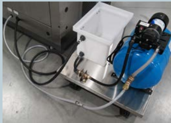
System has a recirculation mode and holds 11 gallons
