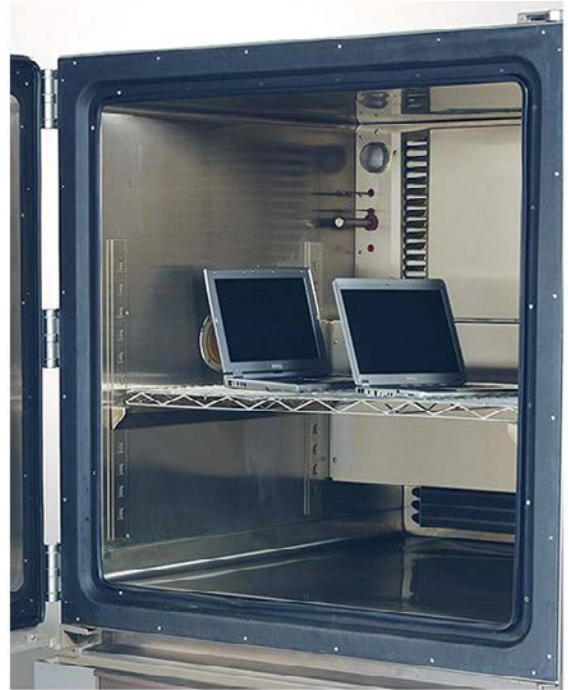
Innovative high-speed airflow suited for fast temperature cycling applications.
