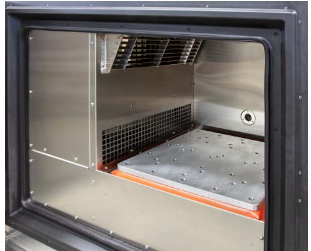
EQZ4 interior with 18" x 18" repetitive shock table
