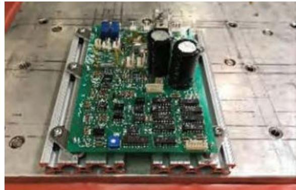
Fixture kits are cost-effective set of parts for mounting your samples on ESPEC's repetitive-shock vibration tables.
