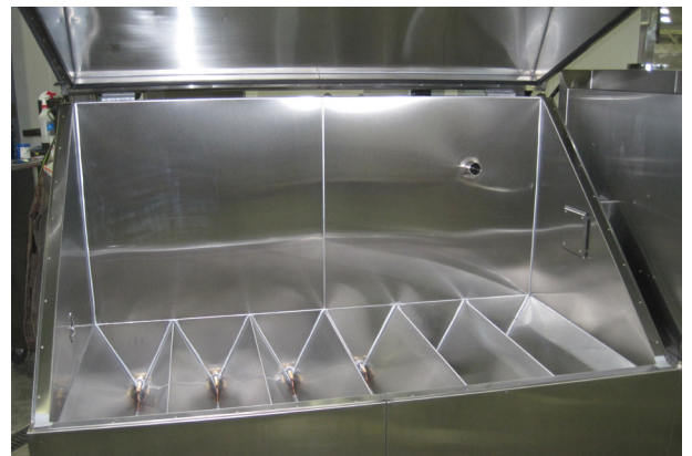
The W-shaped hopper collects the dust after agitation. (Shown without the mesh shelf installed.)
