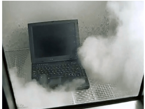
Settling dust chamber starting an agitation cycle.
