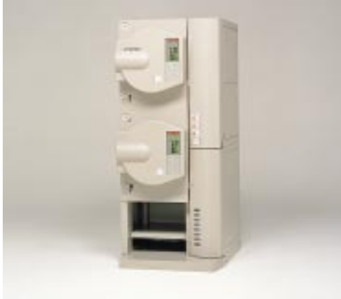
Photo 1 HAST Chamber (Highly Accelerated Stress Test Chamber), product of Tabai Espec
