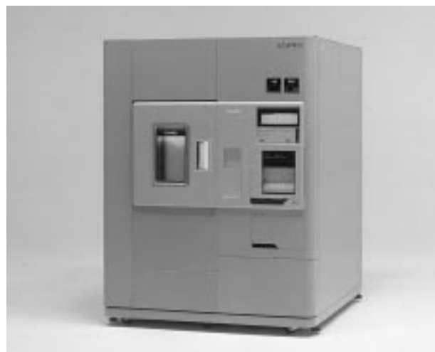
Photo 1 Dew Cycle Test Chamber (Model DCTH-70, produced by TABAI ESPEC)
