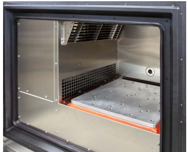
EQZ4 interior with 18" x 18" repetitive shock table
