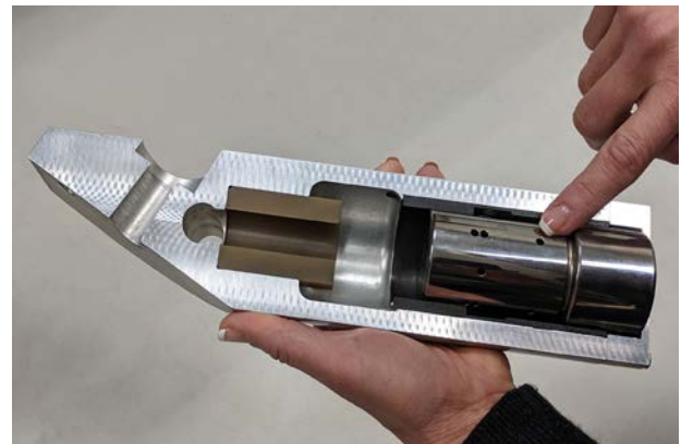
The repetitive shock actuator is a pneumatic hammer that repeatedly impacts the table to create random vibration stress to your test sample.
