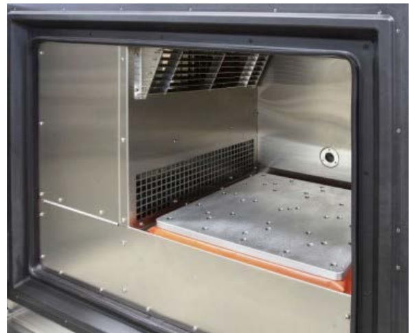
18"x18" vibration table with Qualmark repetitive shock technology.
