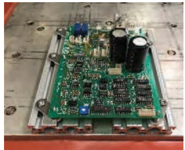
Optional PCA fixture kits are easy-to-use mounting hardware for your electronics to the table.
